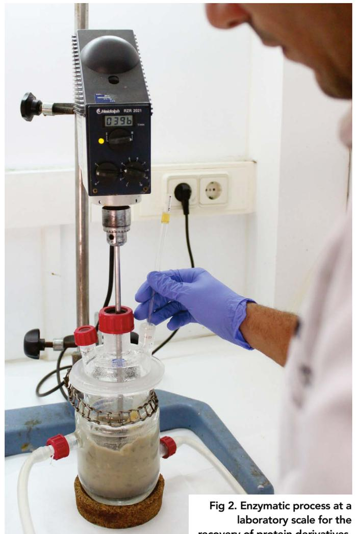
Fig 2. Enzymatic process at a laboratory scale for the recovery of protein derivatives.
